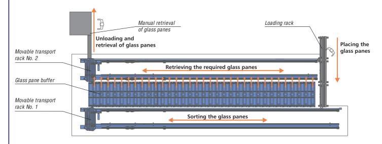
Example of a station: Automatic transfer of panes to an automatic glass pane gluing machine of type GVA115
