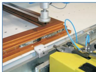
The bolting unit consists of an automatic bolting device complete with a bolt sorting and singularising device for one type of bolts. The automatic bolting device is mounted on an easy-glide guide for convenient positioning.
