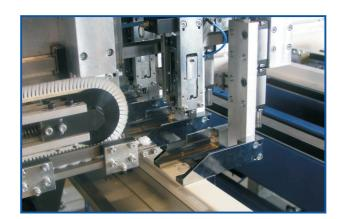
At the mounting station, the mounting head takes up in one operation all the clips that are required for the element to be machined. At the same time the frame is fed in via felt-covered belts and clamped. The mounting head is positioned at the respective frame piece and sets the clips. The number of clips to be attached at the same time depends on the number of setting units that thus define the machining time.
